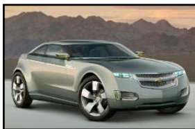
Chevrolet Volt Extended Range EV 40-mile EV range 16kWh Li-Ion
